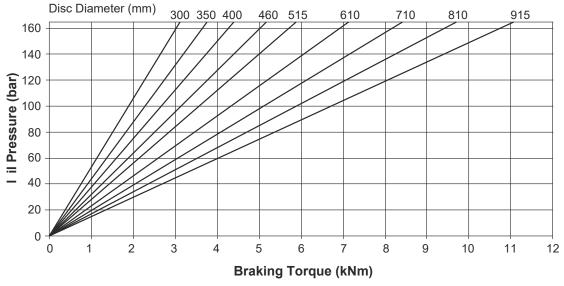
The ratings shown on the above graph are based on fully bedded and conditioned brake pads with nominal friction coefficient  $\mu$ =0.4.
