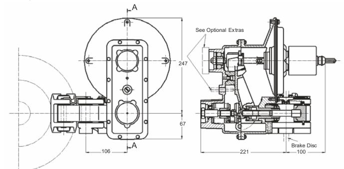
3 off Caliper mounting bolts M12 grade 8.8 and nuts grade 8, tightening torque 80 Nm - Not supplied with caliper
