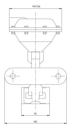
Weight (caliper and thruster) - 2.8kg (thruster only) - 1.3kg
