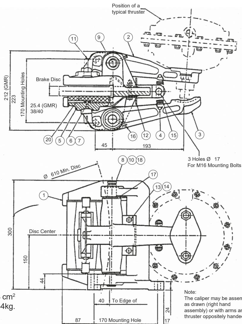
**GMR Caliper Assembly Part Number 6780971 - GMR40 Caliper Assembly Part Number 6781006**
